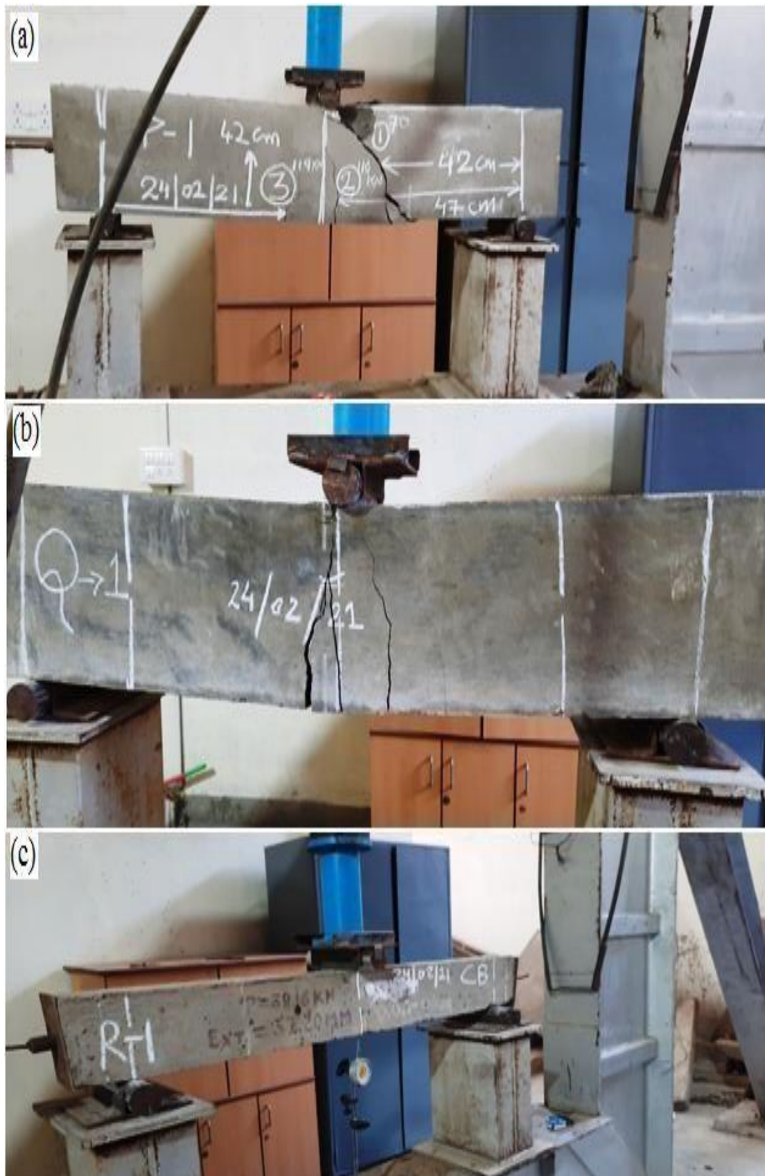
Figure 4.3 shows the crack pattern for (a) Beam P-1 (b) Beam Q-1 (c) Beam R-1
