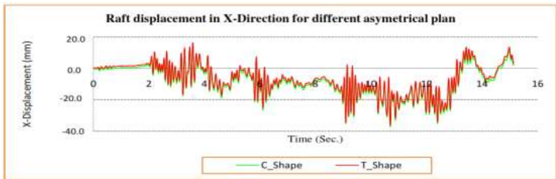
Figure 4. 78 for a typical pile structure at a crucial corner, the X-direction displacement of the raft over time for various asymmetrical forms
