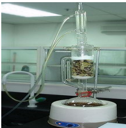
Fig 29: Soxhlet Extraction process of Shewaga
