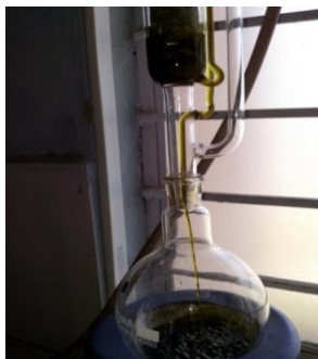
Fig. 30: Soxhlet Extraction process of Tulsi
