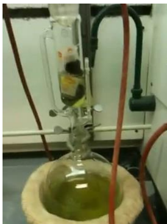
Fig 31: Soxhlet Extraction process of Neem
