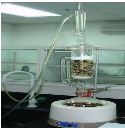
Fig 29: Soxhlet Extraction process of Shewaga
