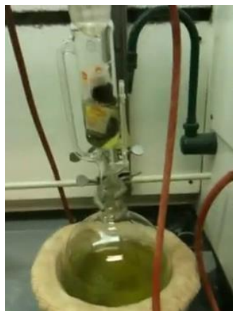
Fig 31: Soxhlet Extraction process of Neem
