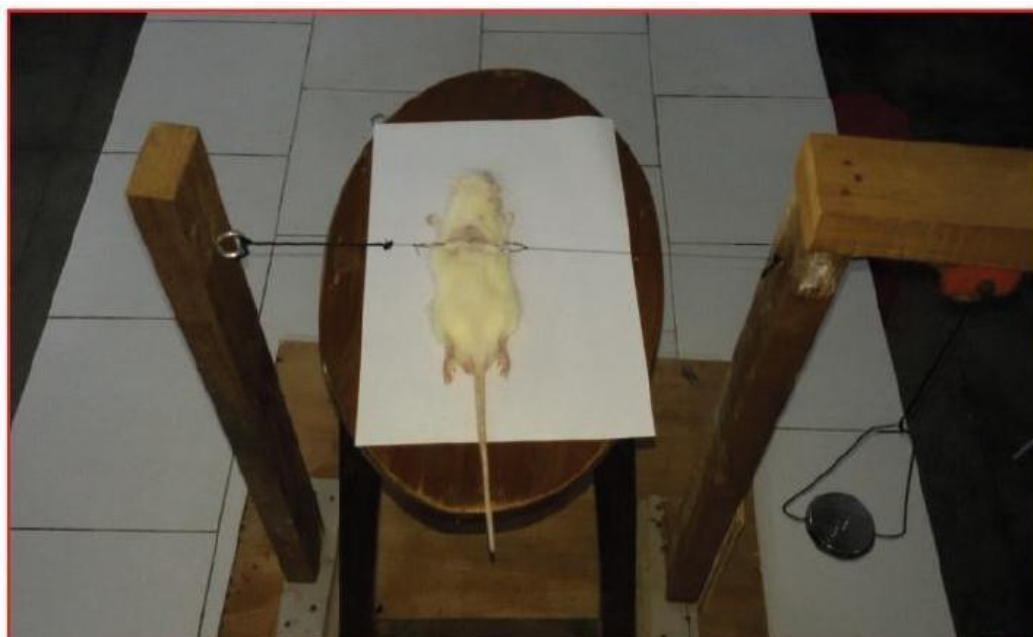
Fig.83: Tensiometer: for the measurement of tensile strength
