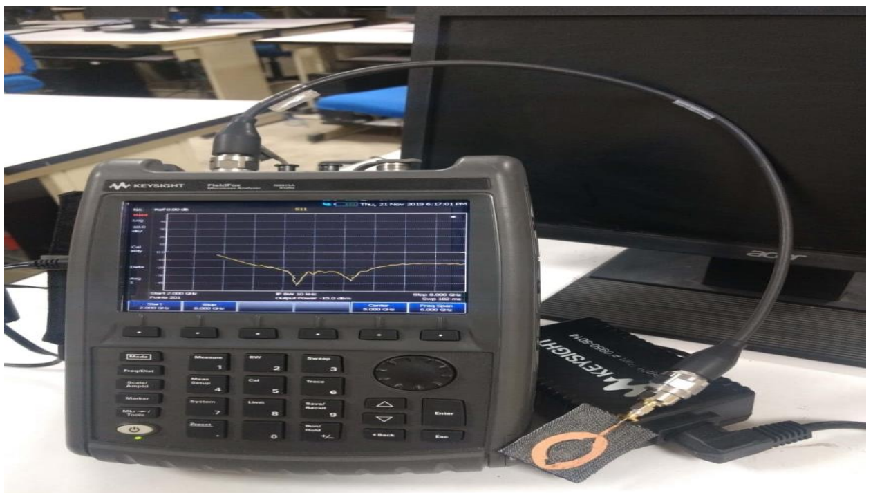
Figure 6.7 Setup for measuring reflection coefficient of proposed antenna-2
