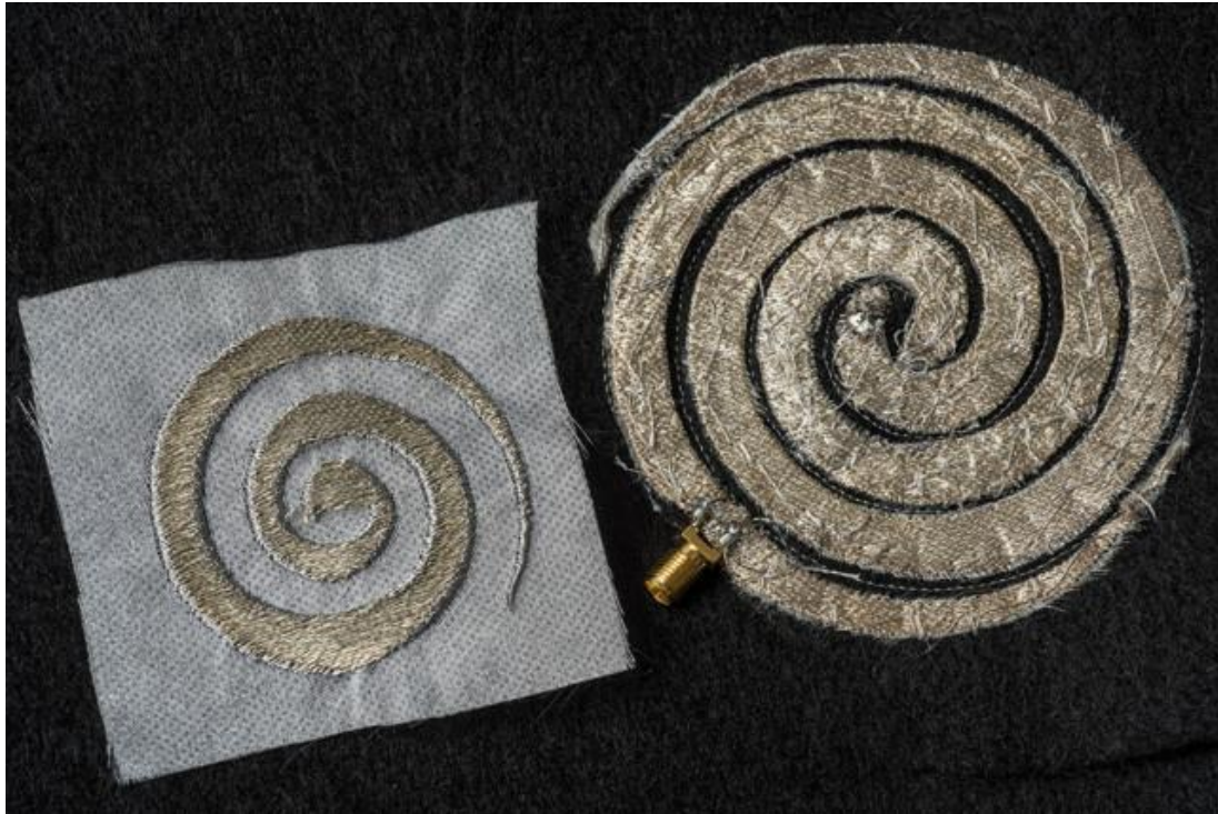
Figure 6.1(b) Stitched Textile Antennas
