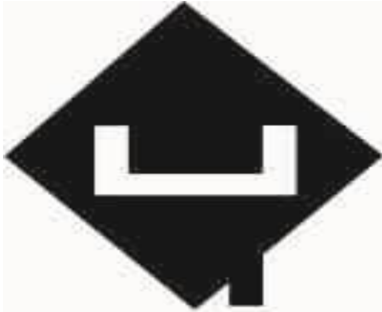
Figure. S.3 : printed structure of the Antenna After Slots
