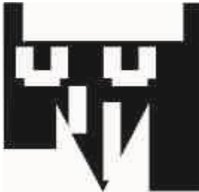
Figure. 4.17: 3D Geometry of the Antenna After Slots Etched Out
