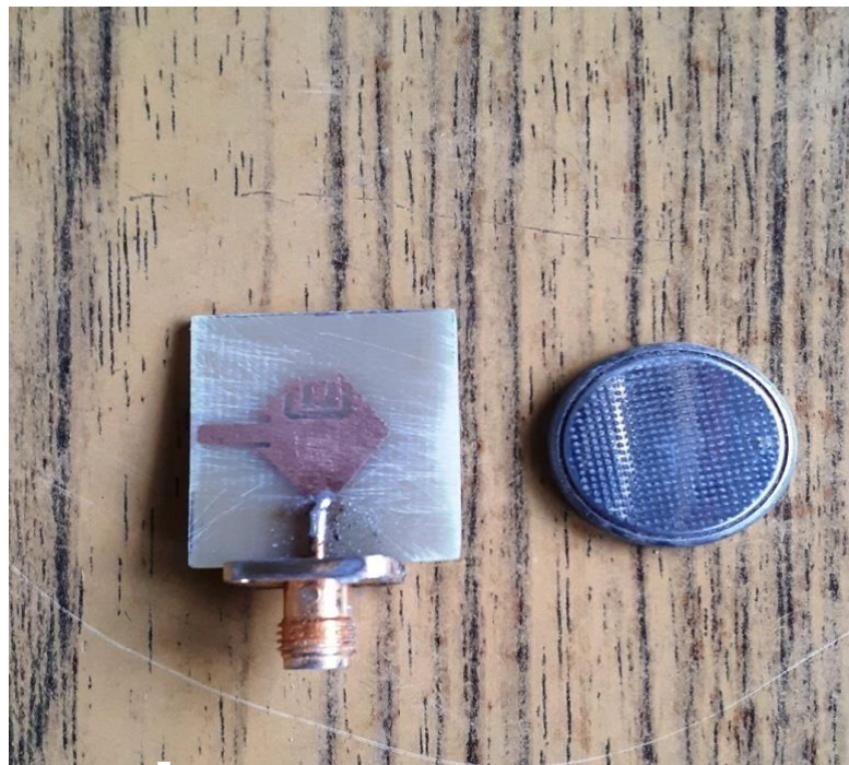
Figure S.16 : Hardware Size Comparison (Button cell) of Proposed Novel Shape
