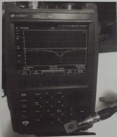
Fig. 6: S 11 (Return Loss) Vs frequency of microstrip antenna on Vector analyzer
