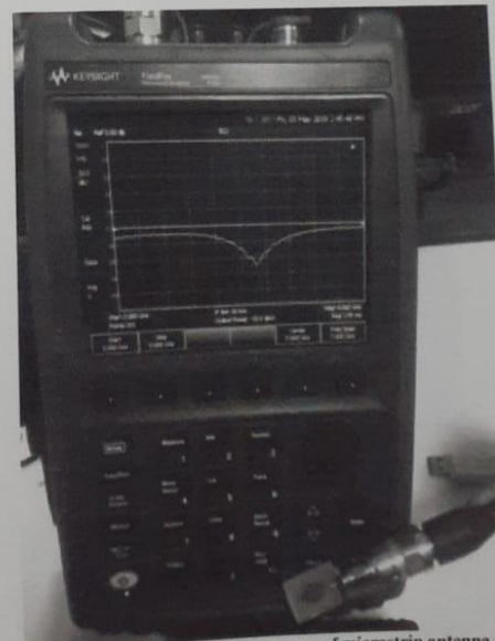
Fig. 6: S_{11} (Return Loss) Vs frequency of microstrip antenna on Vector analyzer for shape 1
