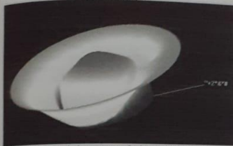
Fig. 21: 3D radiation pattern of microstrip patch radiator shape 2
